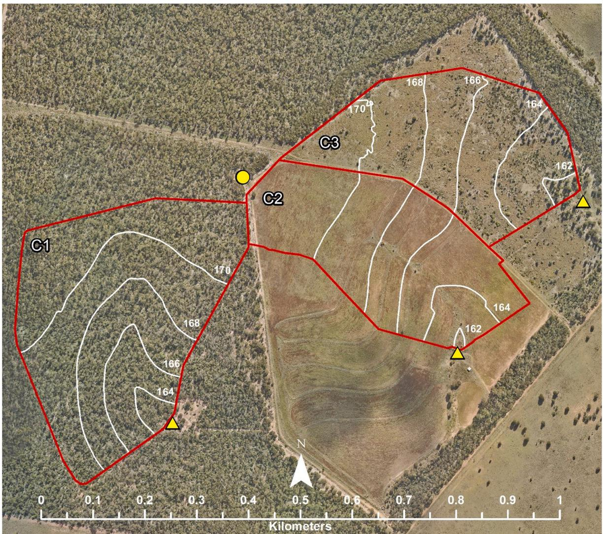
Fig. 1. Aerial photograph of the Brigalow Catchment Study showing catchment boundaries, topography and the location of monitoring equipment. The tipping bucket rainfall recorder at the head point of the catchments is indicated by the circle icon while runoff recording stations are indicated by the triangle icons. Spot heights are in metres.
