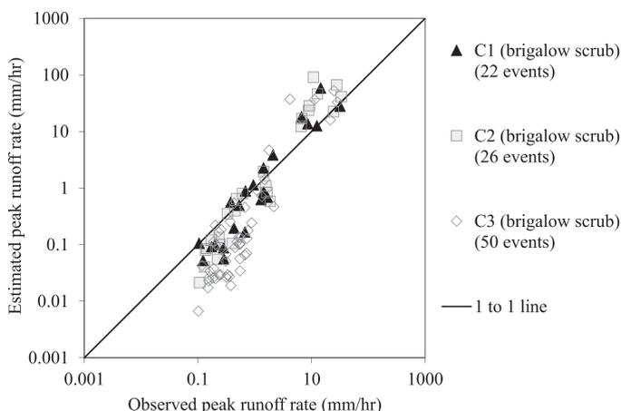
**Fig. 6.** Observed peak runoff rate compared with peak runoff rate estimated using the NRCS method for the three catchments during Stage I.
