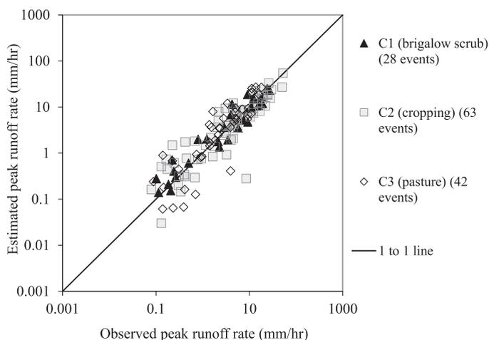
Fig. 9. Observed peak runoff rate compared with peak runoff rate estimated using the VIR method for the three catchments during Stage III.
