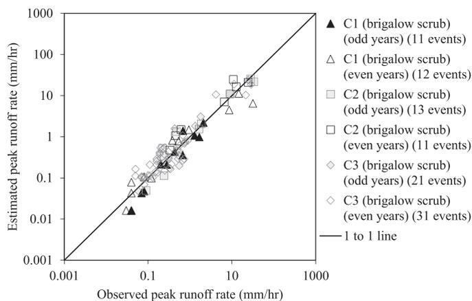
Fig. 2. Observed peak runoff rate compared with peak runoff rate estimated using multiple regression model equations (Table 2) for the three catchments during Stage I.
