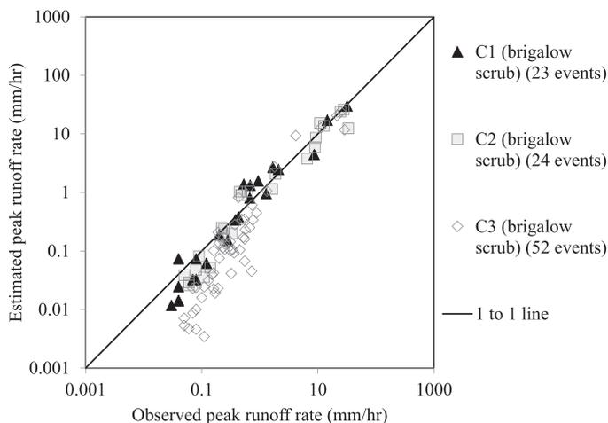
Fig. 4. Observed peak runoff rate compared with peak runoff rate estimated using the scaling technique for the three catchments during Stage I.
