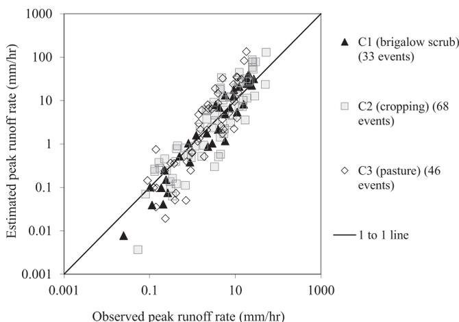
**Fig. 7.** Observed peak runoff rate compared with peak runoff rate estimated using the NRCS method for the three catchments during Stage III.
