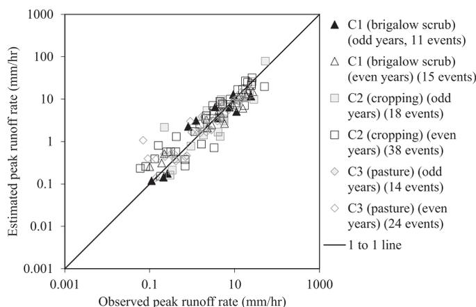
Fig. 3. Observed peak runoff rate compared with peak runoff rate estimated using multiple regression model equations (Table 2) for the three catchments during Stage III.
