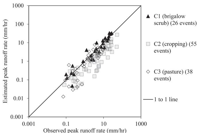
Fig. 5. Observed peak runoff rate compared with peak runoff rate estimated using the scaling technique for the three catchments during Stage III.
