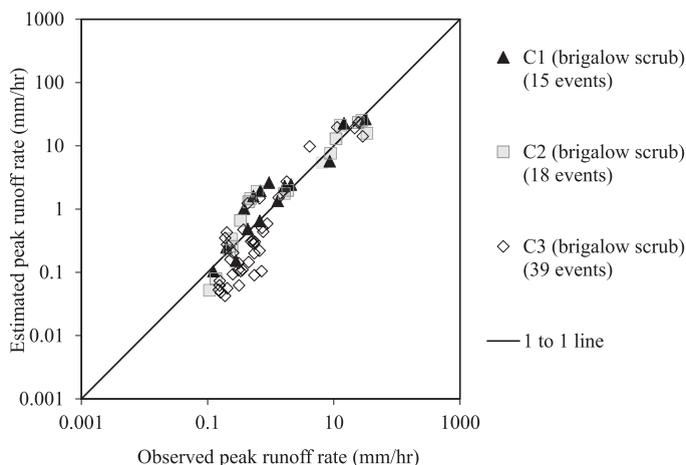
Fig. 8. Observed peak runoff rate compared with peak runoff rate estimated using the routed VIR method for the three catchments during Stage I.
